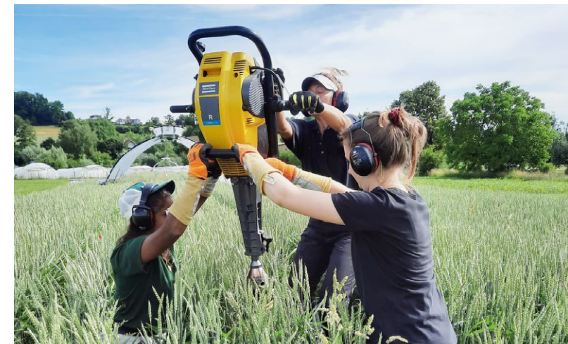
Soil sampling in the DOK long-term trial with the pneumatic soil corer Cobra in Therwil, Switzerland, during wheat flowering (Jennifer Michel, University of Liège, researcher; Marie-Elise Gonzales, FiBL, intern; Sandy Manfroy, University of Liège, researcher).
