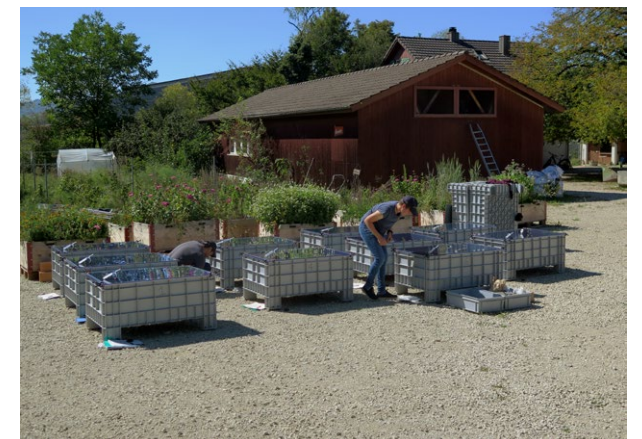
Experimental setup for measuring emissions of greenhouse gases and ammonia from duckweed grown on diluted slurry.
