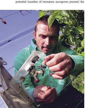
The weather station requires careful maintenance in order to deliver reliable data. The photograph shows Christophe Suter exchanging a piece of blotting paper which simulates leaf wetness.
