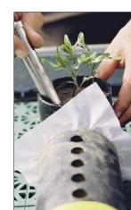
This testing system makes it possible to quantify nutrient intake through mycorrhizal hyphae.
